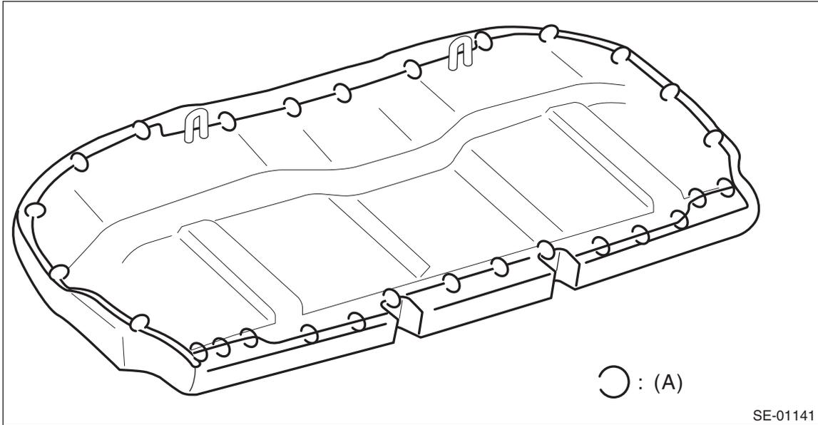
13) Remove the hog rings (A), then remove the seat cushion cover.
