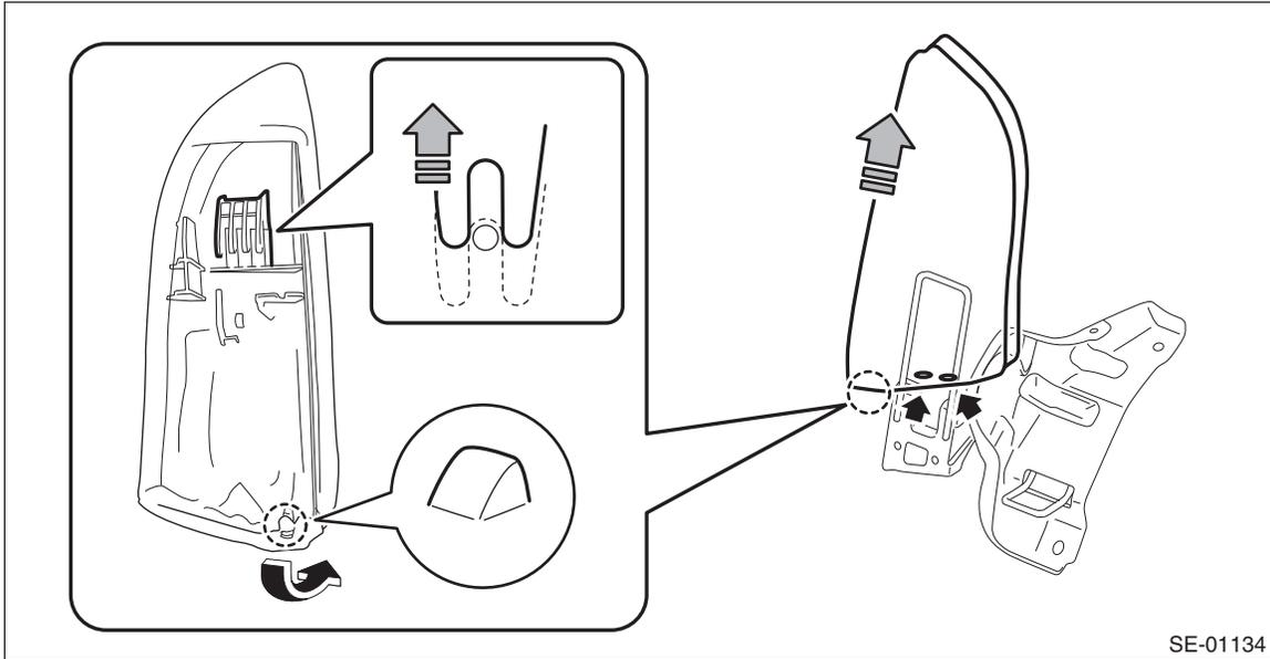
5) Referring to the above steps, remove the backrest side pad assembly LH.
