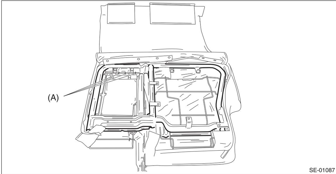
8) Remove the hog rings (A) on the front side of backrest, and then remove the backrest cover.
